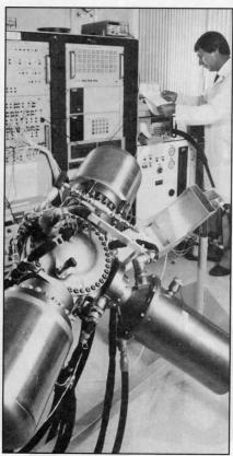
Hughes' Vuilleumier-cycle cryogenic cooler passed an accelerated five-year test to simulate space applications.
