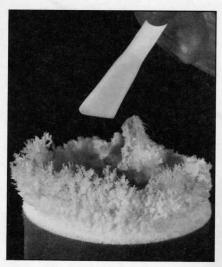
GTE Laboratories' chemical vapor purification process produces crystalline particles of zirconium fluoride that are 90 percent purer than those made by current methods. When fully developed, fluoride optical fiber is expected to transmit information 20 times farther than is possible with present fiber.
