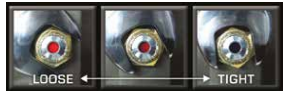
The SmartBolts indicator turns from red to black when proper tension has been reached and is reusable for the life of the fastener
