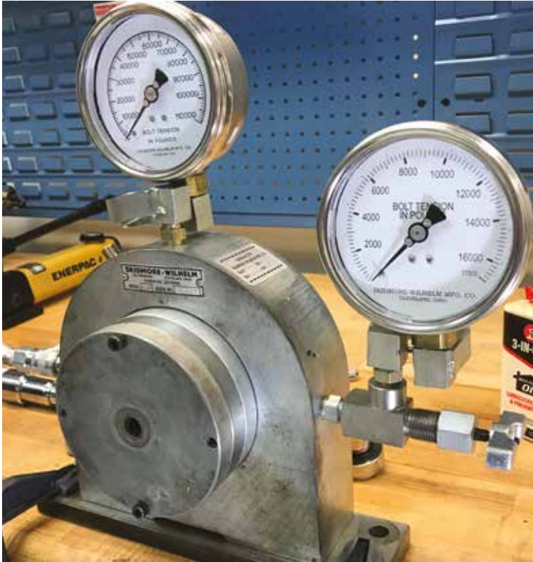
By applying the specified torque to the bolt in the load cell, you can mimic the bolted joint as closely as possible and see how much tension is developed
