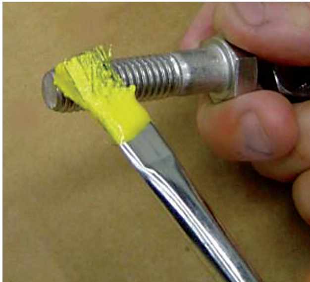
Lubrication affects the friction of the system and this in turn affects the amount of torque required to securely tighten the bolt.
